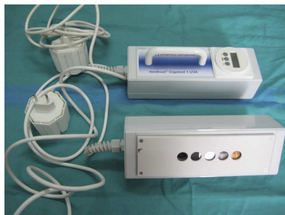
Figure 4 Portable fluorescent hand lamp. A 9-W continuous-spectrum lamp (PLS Special model) with integrated emission spectrum filter, five 5-mm test fields that emit 7%, 34%, 63%, 85% and 100% of the UV-B or UV-A spectrum and therefore make it possible to calculate the exposure dose (in J/cm^2 ) as a function of skin contact time (Gigatest, Medisun, France).
